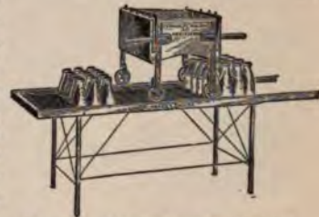
Fig. 246. Side-bar milk-bottle filler.
